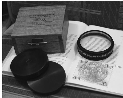
This report is unusual as it combines several observations made during the hot summer of 2015. All four nights had in common the telescope – long oil doublet 82/1670mm of my own design, and the targets – small bright planetary nebulae. This tiny lens revealed an interesting level of details in all cases.
