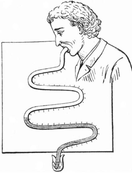
**Fig 3.** Thermoscope invented by Professor Santorius, serving for determination of “*temperatura*” of human body, about 1612. Instrument was made of glass and filled with wine. The bulb having diameter of golf ball was during the measurement inserted into patient’s mouth.
