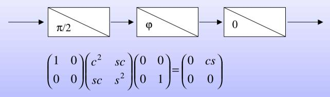
If this sequence is applied on a linearly polarized beam:
